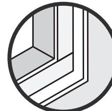
Apply your White 13mm Standard metal tape as close to the frame edge as possible.
