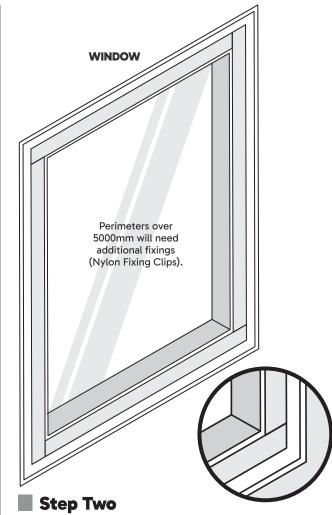
Find your White magnetic tape firstly and cut to the appropriate lengths for applying to the window frame (remove backing tape). A pair of scissors or a craft knife are ideal for this purpose. Your magnetic tape will either be 13mm or 25mm wide depending on your panel size and kit.
