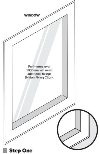
Unpack your acrylic pane(s) and magnetic tapes, check that they are intact. Ensure you have a flat table or surface beforehand when applying your magnetic tape to your acrylic pane(s). This will avoid any bowing or warping and ensure a tight seal.
