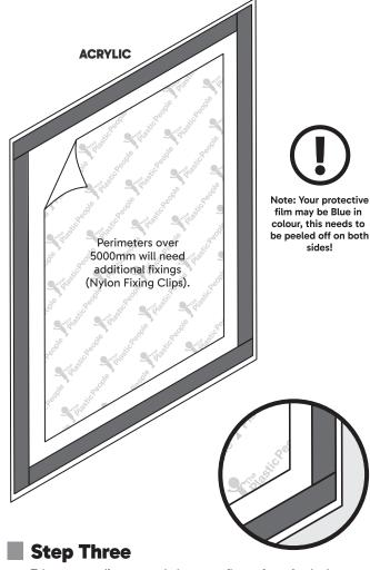
Take your acrylic pane and place on a flat surface. Apply the Black magnetic tape around the outer edge of the acrylic side that has the film partially removed (remove backing tape). Once completed take off the protective film in the middle. Leave protective film on reverse of your panel until you apply to your window.
