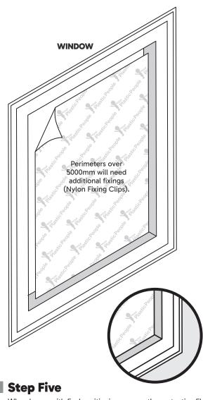
When happy with final positioning remove the protective film from the front, peeling carefully. Ensure your seal is good and secure and run your fingers around the outer aspect.
