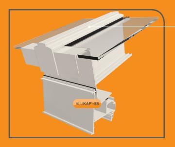
16. Now carefully cut the ALUKAP®-SS Top Bar Top Cap to the accurate length required for a perfect aesthetically pleasing finish. For gable end or wall abutments use the ALUKAP®-SS Gable Bar or Wall Bar Top Cap. Snap the ALUKAP®-SS Top Bar Top Caps on to the ALUKAP®-SS Top Bar Base Caps along the whole length of the bar. Use a suitable rubber / plastic headed hammer for this action and avoid heavy impact, to avoid damage to the ALUKAP®-SS bar and the glazing materials.
