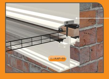
18. Fit a flashing tape or lead to the back wall and any adjacent wall as required
